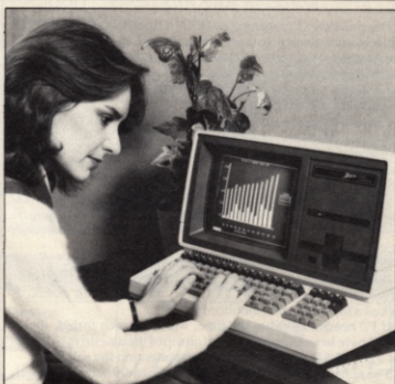
ZENITH DISKS — Zenith has added hard disk options to its Z100 range of business micros. Pictured is the 'all-in-one' ZW120, with 10Mb Winchester and 320K floppy. There's also a 'low profile' ZW100 for use with a separate colour or green screen monitor. The new machines come with 192K user RAM plus the usual Z100 specs of 8085, 8088, $100 bus, CP/M, Z-DOS (MSDOS) and Z-Basic. Prices for the hard disk machines start from a competitive £3,925. Zenith is in Gloucester (0452) 29451.
